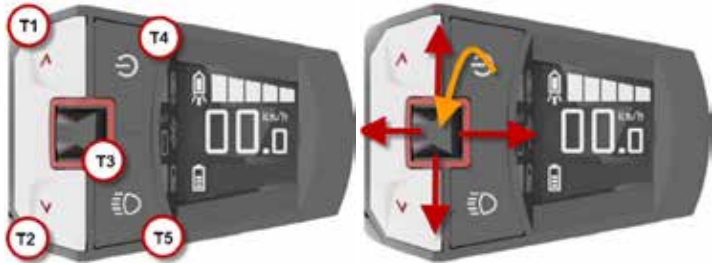
Fig. 1 Keys and joystick of the Comfort control unit (figure shows left-hand installation. The display and function of the keys are mirrored when mounted on the right-hand side). Shown amount of support levels and battery indicators may vary due to your system configuration.
